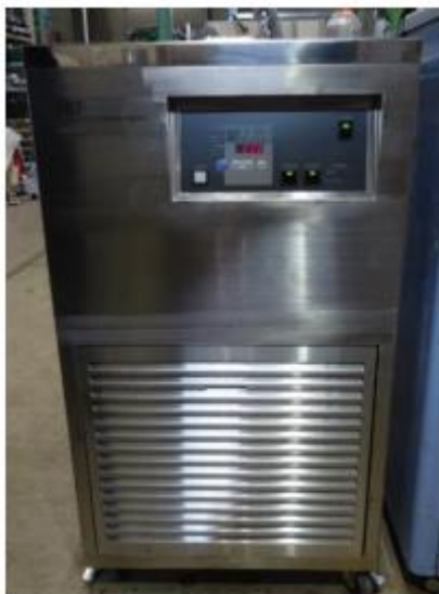
Figure 2.18. Heat source water supplier
