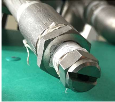
Fig. 4-5 Air mist spray nozzle tip.
