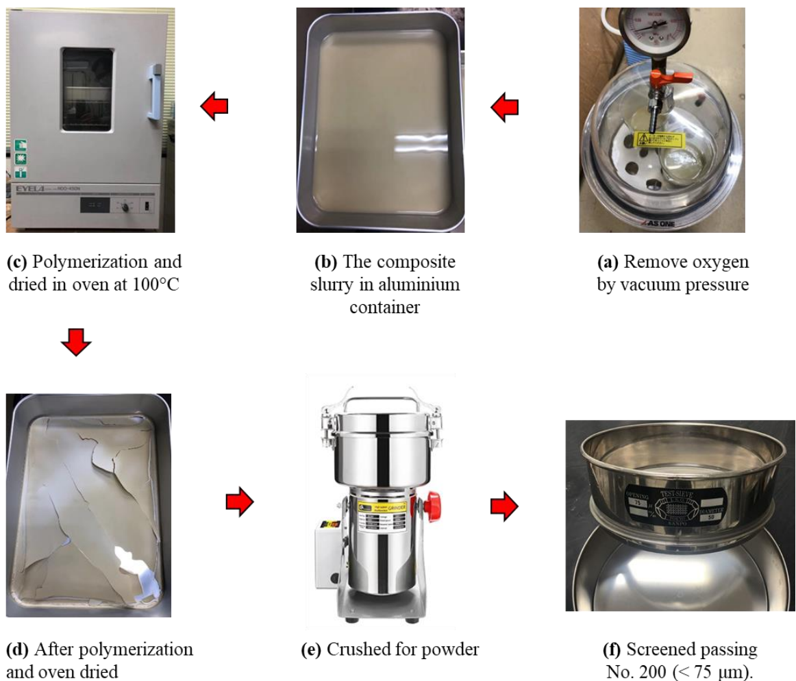
Fig. 3.4 The process of producing PB
