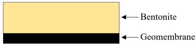
Fig. 1.4 Cross section of GM-GCLs (modified from (EPA 2017))
