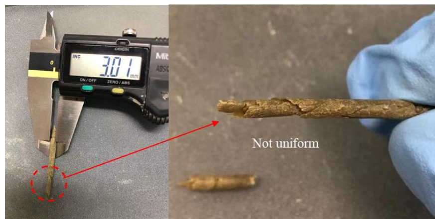
Fig. 4.1 The sample of 0.1PB in plastic limit test.
