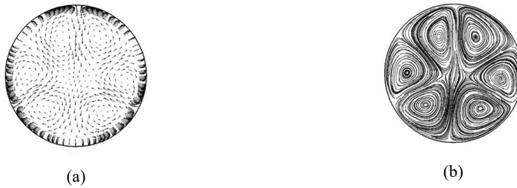
Figure 2.9 Cross-section flow structure in the modification of DDIR-tube (a) velocity vectors, (b) streamlines (Zheng et al., 2020)
