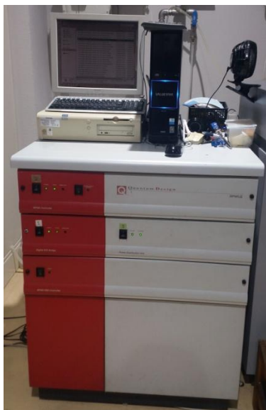
Figure 2.6. Photograph of the magnetic property measurement system (MPMS) based on a superconducting quantum interface device installed at Low-Temperature Center, Applied Physics and Quantum Computation Science department in Kyushu University that was used to measure the present studied compounds.
