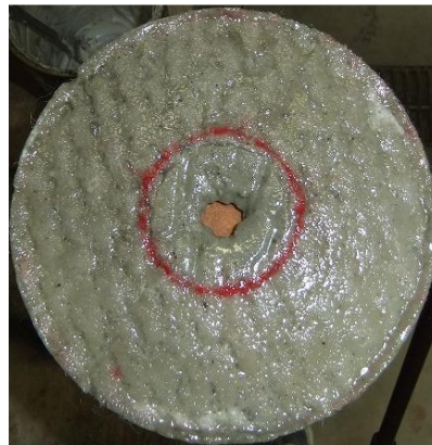
Fig. 2.16 Photo of healed GT-GCLs after tests (after Sari, 2013)
