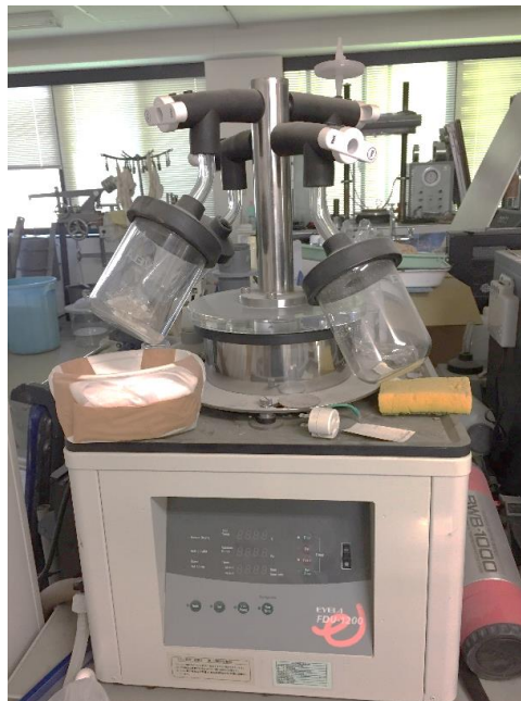
Fig. 3.21 Freeze dryer machine
