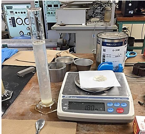
Fig. 3.12 Free swelling index test
