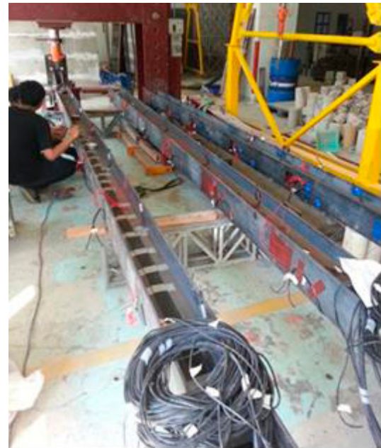
Fig. 3. Strain measurements by affixing strain gauge on steel surface.
