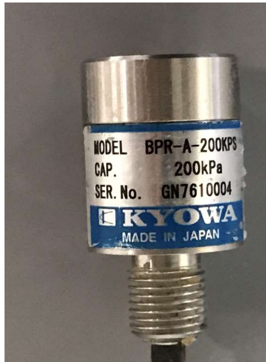
Figure 3.2 Pore pressure transducer used in model test
