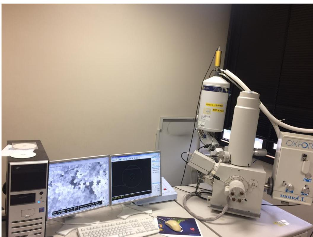
Figure 2.6 The appearance of the SEM equipment.
