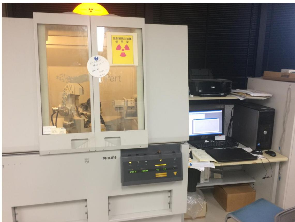
Figure 2.4 The appearance of the XRD equipment.
