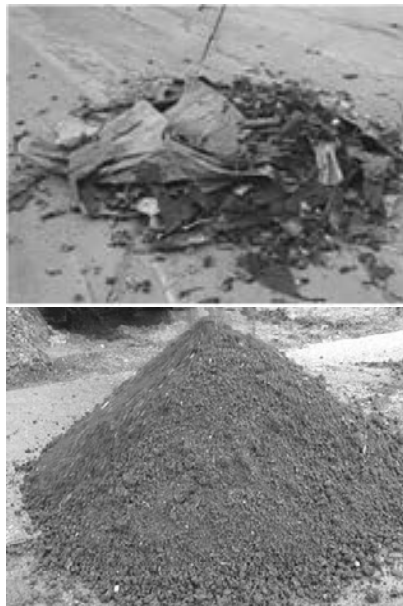
Photo 20 Case 2: Rubble and disposed soil (added 5% of quicklime)
