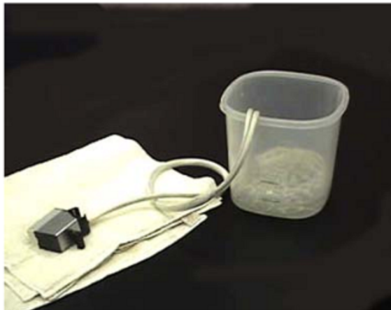
Figure 4.6: Soaking arrangement of the sensor array in the electrolyte bucket
