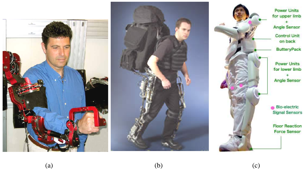
Figure 2.1: Different types of Exoskeletons (a) CADEN)-7 : Upper-Limb [7] (b) Berkeley Lower-Limb [8] (c) HAL full body exoskeleton [9]
