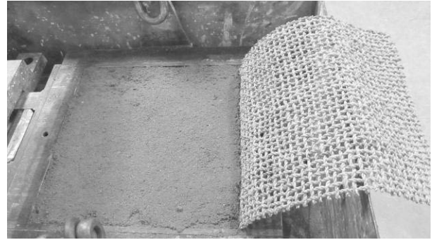
Fig. 8 Kenaf LLGs folded with sand backfill in shear box
