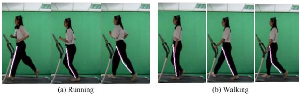
Figure 3-4: Leg motion extraction results of running and walking by temporal template matching in [25]
