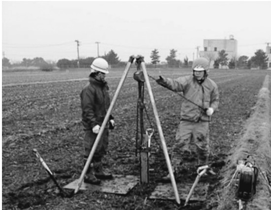
Fig.7 Soil sampling by using a "Handy Geoslicer"
