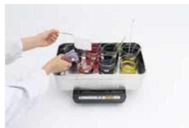
Fig. 25.25 Remove the fibre, add the dye, mix well and reinsert the fiber.
