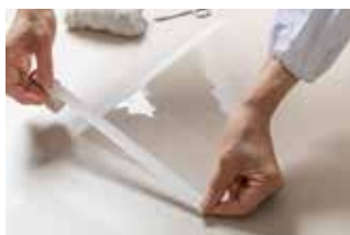
Fig. 24.3 Wipe the water around the sheet and secure it with masking tape.
