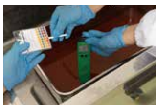
Fig. 8.19 Extract carthamin with alkali
