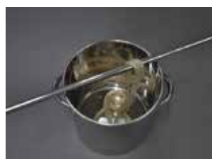
Fig. 8.9 Passing a rod between the loop during dyeing prevents the yarns from tangling.
