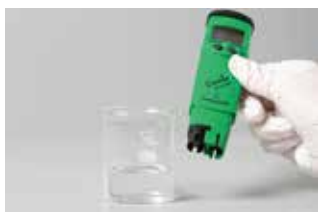
Fig. 18.5 A pH meter measures hydrogen ion concentration with an electrode.
