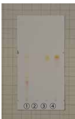
Fig. 10.1 TLC Dyer's madder (Day light photography)
