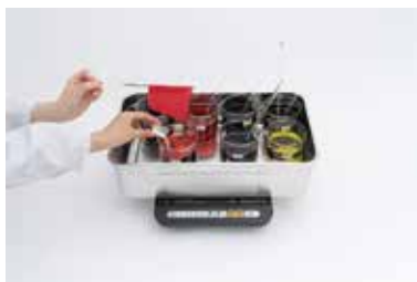
Fig. 25.26 Remove the fibre, add the auxiliary agents, mix well, and reinsert the fibre.
