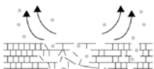
Fig.14.5 Since the degraded fibres are decomposed, they do not swell and they collapse when water enters.
