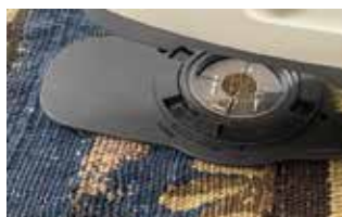
Fig. 9.4 Measuring the surface colour of the threads.
