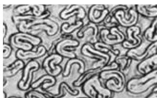
Fig.5.9 Cross section of cotton fibres. In the centre is a hollow lumen. (AATCC)
