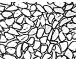
Fig. 5.27 Cross-sectional structure of scoured silk without sericin, the triangular shape of fibroin can be seen independently. (AATCC)
