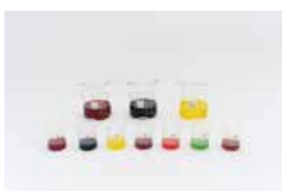
Fig. 25.11 Measure and combine the stock solution by calculating the depths of shade, and amount of dye according to the weight of fibre.
