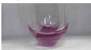
Fig.9.13 Cochineal fabric in ammonia (pH12) Change
