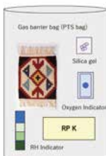
Fig. 11.72 Place the agent, silica gel and oxygen indicator in the Escal film.
