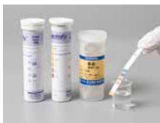
Fig. 18.3 Water quality inspection using various test papers.
