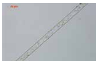
Fig. 5.33 Polyester fibre 400x (CAMEO)
