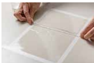
Fig. 24.4 The thickness of the adhesive film is adjusted by layering masking tape, and the adhesive is stretched with a glass rod.
