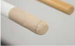
Fig. 11.6 Wooden rods are painted with an acrylic coating and covered with fabric
