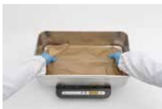
Fig. 25.19 While dyeing spread the fabric and constantly move it towards the front and back.
