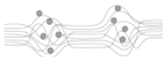
Fig. 7.5 Dyeing mechanism: migration of dyes in the amorphous regions of the fibre.
