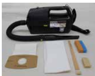
Fig. 16.1 HEPA filter vacuum cleaner, bag, nano-fibre wiping cloth, soft brush, latex sponges
