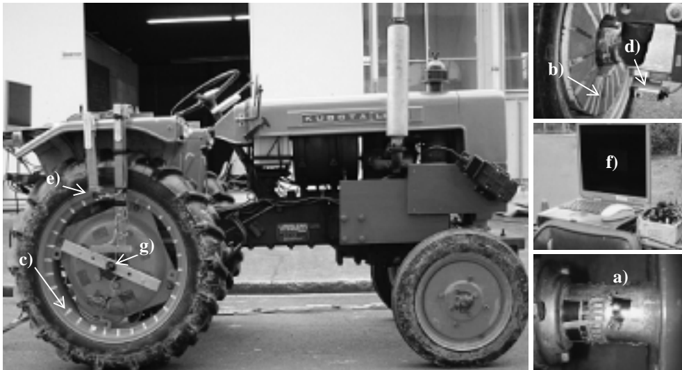
Fig. 4. Tractor instrumentation: a) strain-gage based transducers; b, c) reflective tapes; d, e) photo switches; f) data acquisition system; g) slip ring
