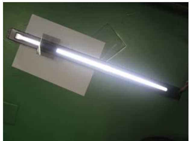
Fig.6 Light source used (20W three wavelength combined quasi natural light source with polarization film)
