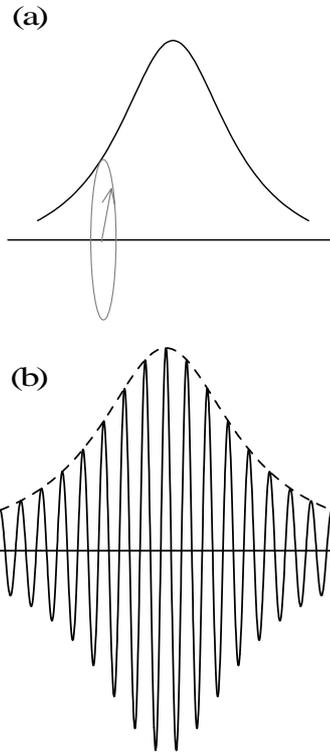
Fig.9 Quantum wave function and modulated carrier wave
