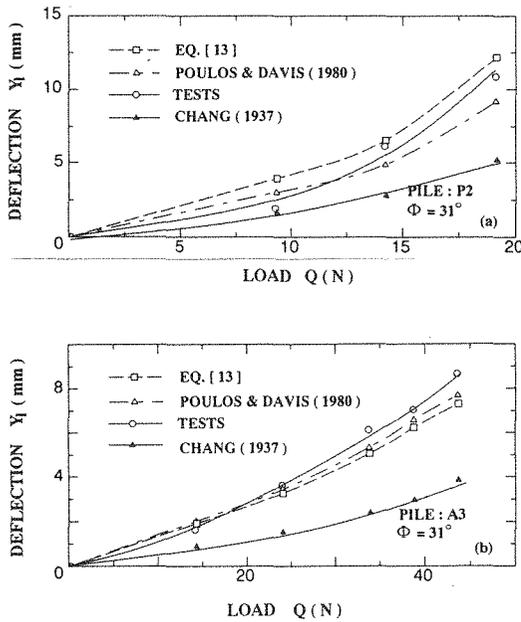
Fig. 7 Relation Between Load Level Horizontal Deflection  $Y_1$  and Load  $Q$ , for (a) Pile P2 (b) Pile  $A_3$ .
