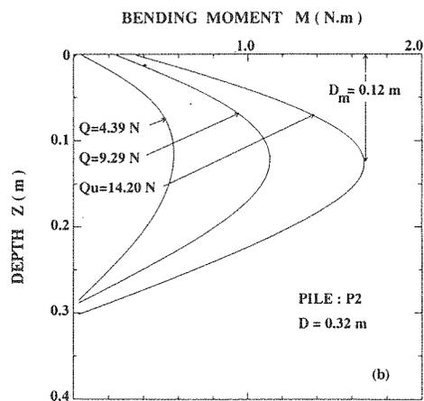
Fig. 4b Variation of Bending Moment With Depth and Load for Pile P2.
