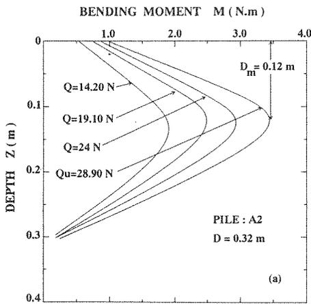
Fig. 4a Variation of Bending Moment With Depth and Load for Pile A2.
