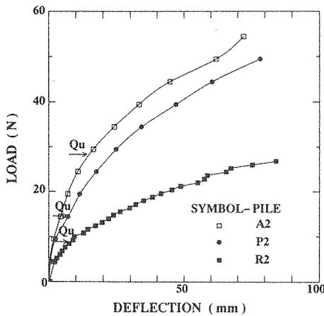
Fig. 2 Typical Load Deflection Curves.
