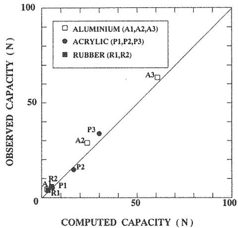
Fig. 3 Computed and Observed Capacities of the Piles.
