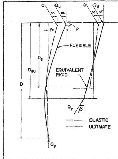
Fig. 8 Schematic Diagram of Flexible and Equivalent Rigid Piles.
