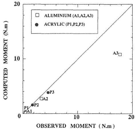
Fig. 5 Computed and Observed Maximum Bending Moments.
