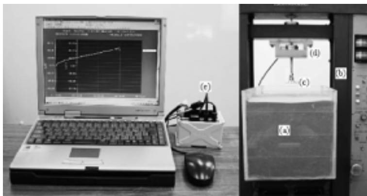
Fig. 1. The sinkage device: a) sand sample; b) loading equipment; c) sinkage plate; d) load cell; e) data acquisition system
