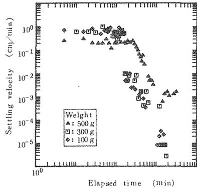
Fig. 12 Plot of settling velocity vs. height for initial weight difference.
