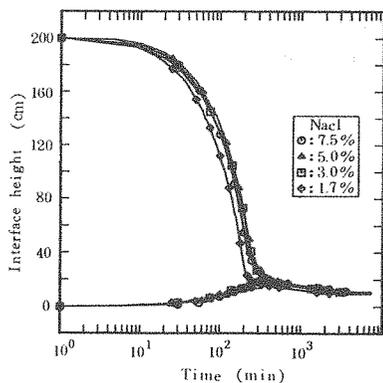
Fig. 7 Settling curve for salinity difference at station C sediment.
