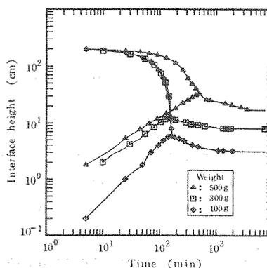
Fig. 9 Logarithmic plot of settling curve as a function of initial weight.
