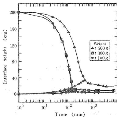
Fig. 6 Settling curve for initial weight difference at station C sediment.
