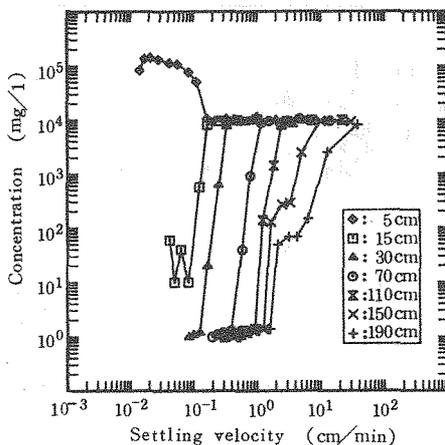
Fig. 22 (a) Relationship between settling velocity ( $w_g = dz/dt$ ) and concentration.
