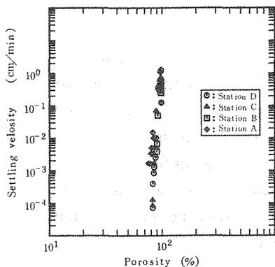
Fig. 14 Relationship between settling velocity and porosity.
