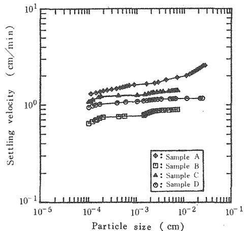
Fig. 23 Relationship between settling velocity and particle size.
