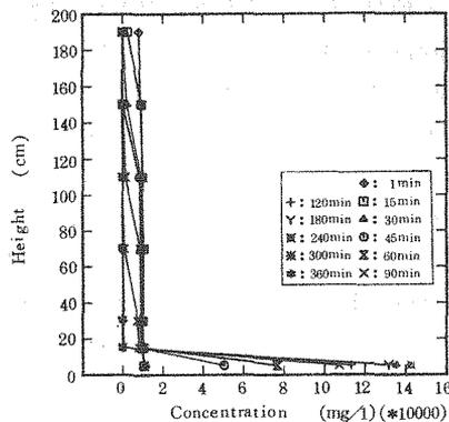
Fig. 18 (a) Variation in the concentration and the height on the station C sediment ( $C_0 = 11,500\text{ mg/l}$ ).
