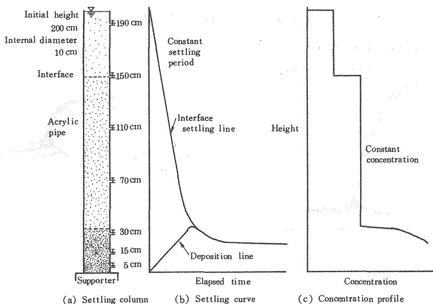
Fig. 4 Schematic drawing of settling column-settling curve-concentration profile.
