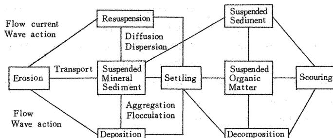
Fig. 1 General model structure of physio-chemical process.
