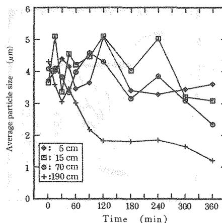
Fig. 21 Variations of average particle size with time for station C sediment.
