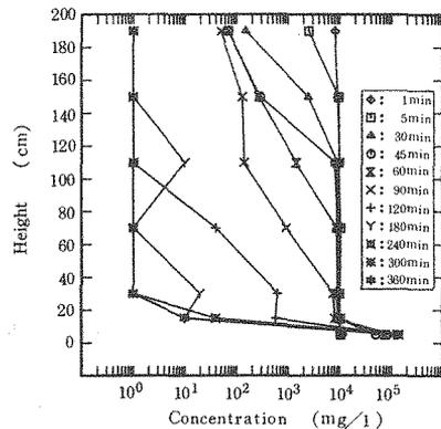
Fig. 17 Variations of concentration with height for station C sediment ( $C_0 = 11,500\text{ mg/l}$ ).
