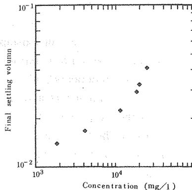
Fig. 15 Relationship between initial concentration and final settling volume.
