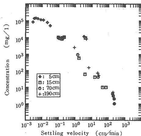
Fig. 22 (b) Relationship between settling velocity and concentration.
