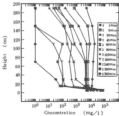
Fig. 16 Variations of concentration with height for station A sediment ( $C_0 = 20,000\text{ mg/l}$ ).
