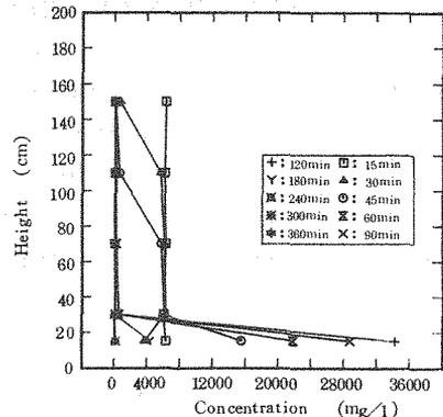
Fig. 18 (b) Variation in the concentration and the height on the station C sediment ( $C_0 = 4,150\text{ mg/l}$ ).
