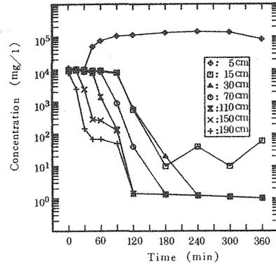
Fig. 19 (b) Variation in the concentration and time on the height ( $C_0=11,500\text{mg/l}$ : Station C).
