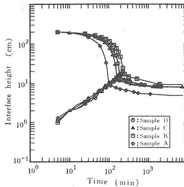
Fig. 8 Logarithmic plot of settling curve as a function of sampling station.
