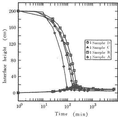
Fig. 5 Settling curve for sampling station difference.
