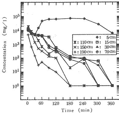
Fig. 19 (a) Variation in the concentration and time on the height ( $C_0=20,000\text{mg/l}$ : Station A).
