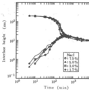
Fig. 10 Logarithmic plot of settling curve as a function of salinity at station C.
